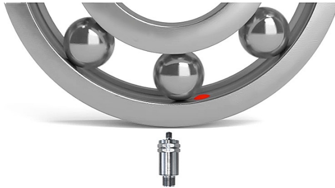
Figure 4. Vibration transducer mounted close to the load zone of a bearing.
